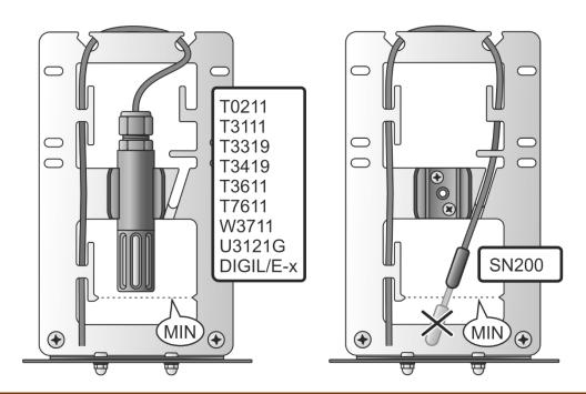
If the probe cable is too thin (approx. 2 to 3 mm, eg for the TG3 probe) and there is a risk of instability of the probe sensor, secure the probe cable by turning the probe holder. See pictures below.
